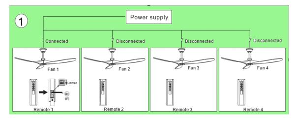
Turn the power supply **on** to all fans and keep all the fans' isolated switches **off**. Turn Fan 1 on and leave the rest off, within 30 seconds, set the DIP switches on Remote 1 to lower position and then press and hold the "SET" button for 5 seconds, **and then again press the same "SET" button for another 5 seconds**. Turn the fan on by pressing the speed button, Fan 1 should operate and is properly set. If not then check the batteries and then try again. NB: Leave the DIP switches down.
