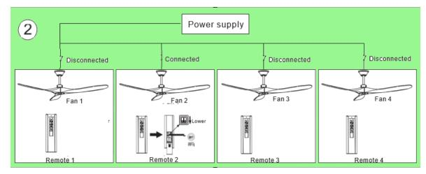
Turn off the isolated switch off on Fan 1, and turn on the isolated switch on Fan 2, keep the rest off. Within 30 seconds, set the DIP switches on remote 2 to lower position and then press and hold the "SET" button for 5 seconds, and then **again press the same "SET" button for another 5 seconds**. Turn the fan on by pressing the speed button, if the fan starts to work then Fan 2 is properly set.
