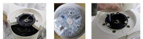
the 3 white washers onto the plate as shown and place the kit onto them – a drop of glue will hold them in place. Locate the screws from the inside of the light kit and using the washer tighten them up.
